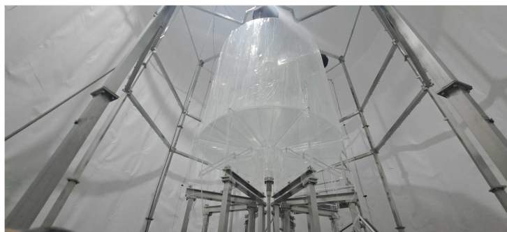
(c) The actual PMT frame together with the central acrylic vessel. Taken during the installation of OSIRIS, Oct. 2022. by T.Sterr
