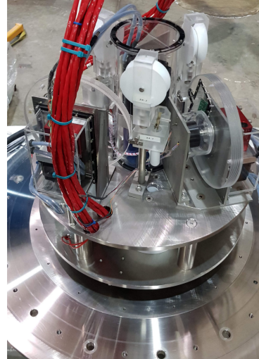
(b) The ACU with removed bell jar. Cables and deploying wheels can be seen. A detailed labeled picture of the inner parts of the ACU can be found in chapter 4.5.1. Picture taken in fall 2022 by Cornelius Vollbrecht.
