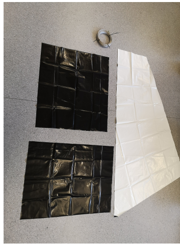
(b) Three exemplary sheets of the optical separation of OSIRIS. All foils will be mounted with the black face pointing inward. At the top, the stainless steel rope used for additional fixation can be seen.
