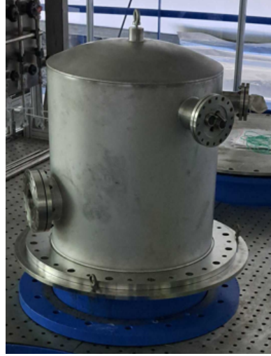
(a) Picture of the OSIRIS ACU as installed in the top clean room of OSIRIS. Visible are the flanges for visual inspection, control and nitrogen (left to right). Picture taken in fall 2022 by Cornelius Vollbrecht.
