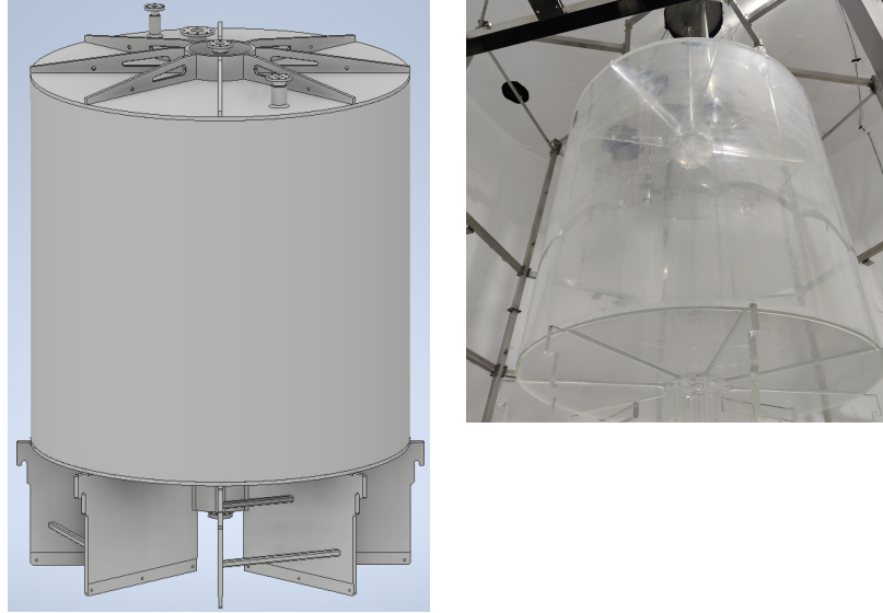
(a) CAD drawing of the central acrylic vessel of OSIRIS. Flanges on top are (from left to right): level measurement, thermometer rod, LS filling and calibration flange.
