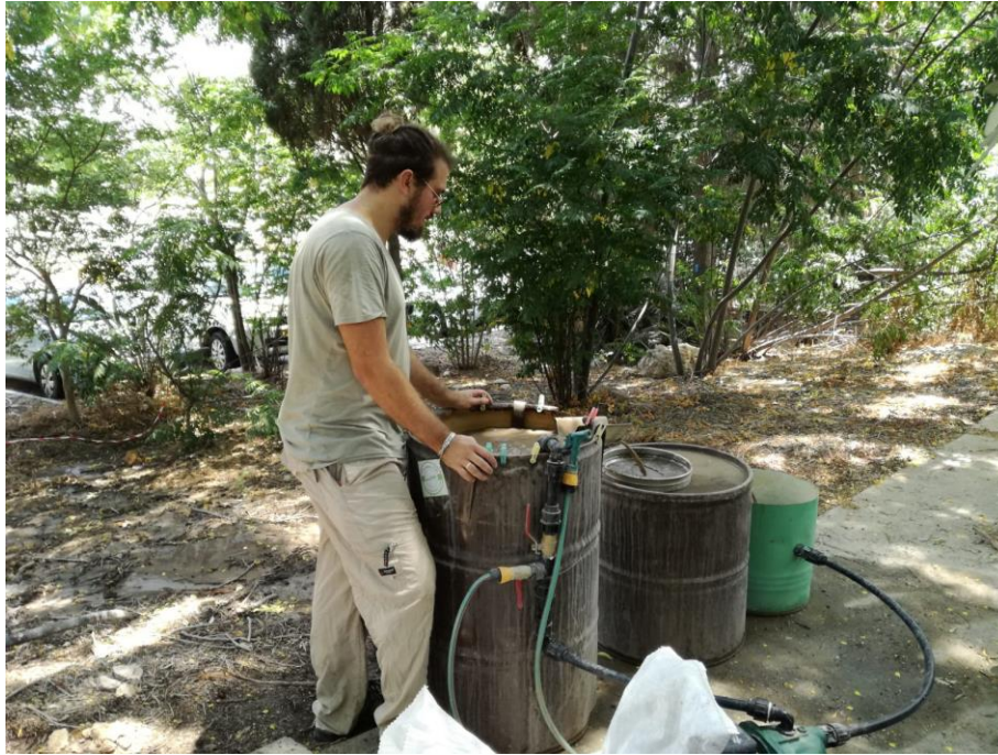
Fig. 5 Flotation machine built and used in loco to process the sediments analyzed in this dissertation
