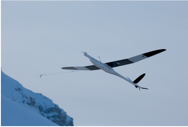
Figure 2: MASC-3 UAS shortly after take-off. The winch cable is still attached to the fuselage. Photo taken at the ISOBAR campaign 2018, courtesy Astrid Lampert
