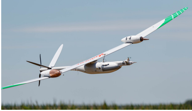
Figure 1.1: MASC-3 UAS (uncrewed aircraft system) shortly after lift-off, equipped with optional wing-pods for particle and electro-static measurements. Photographed by Bernd Lamme for the DWD (German Weather Service). The measurement instruments and probes are located at the very front. To the right, the main technical specifications are summarised.
