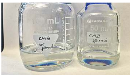
Figure 2.3: First bottle containing CHB brought from sigma Aldrich without being subjected to filtering does not have a yellowish appearance; the second bottle contains CHB after the filter process. Even after storing it for a longer duration, it does not appear to have a brownish color.
