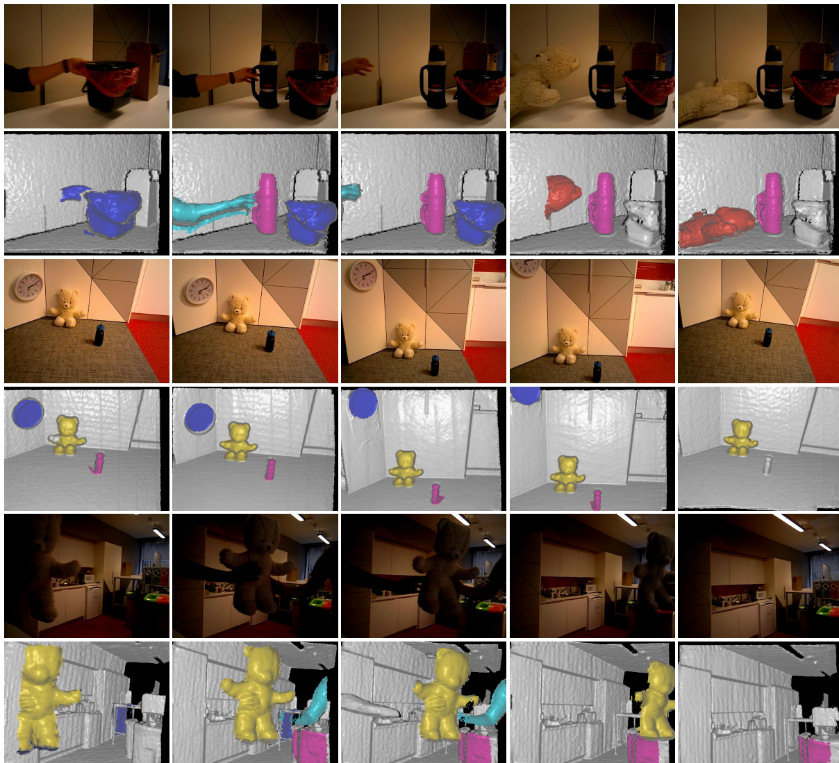
Figure 3.5: Qualitative evaluation on the real-world datasets published with Co-Fusion (Rünz and Agapito 2017). We demonstrate that we can handle fast movement (the second and the third image of the first sequence are only 25 frames apart), as well as objects with relative weak geometric cues, such as the clock in the second scene. Note that the left arm handing over the teddy is not detected in the last scene. While it initially is integrated into the background it is quickly overwritten by actual background depth soon after it moves out of view.
