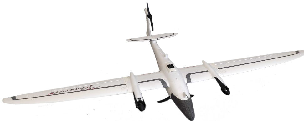
Figure 2.7: The Quantum System Trinity F90+ vertical-take-off drone, which carried the MicaSense RedEdge-MX camera on the data acquisition for the SeadronesSee data set.
