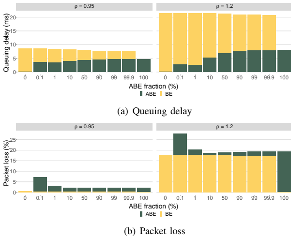
Fig. 10. Queuing delay and packet loss of BE and ABE traffic for non-adaptive traffic with bursts. The relative overall load \rho and the fraction of ABE traffic are varying parameters; other parameters are set as in Table IV.
