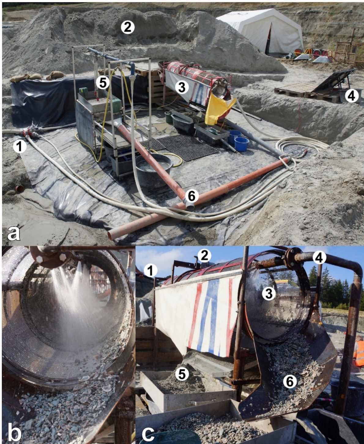
Figure 3.2.2. Fossil screening zone at the early Late Miocene Hammerschmiede locality and the HAM 4 excavation area in 2023. (a1) Water supply by type B and C fire hoses over 700 m from the next hydrant, (a2) piled up sediments, to be washed with (a3) the self constructed rotational sieving system "Rosie", that is powered by a solar panel (a4) with a car battery as buffer storage. The old sieve rack (a5) is used for picking of the washed material. The base of the area is slightly inclined and covered with pond foil and drainage pipes (a6) to effectively drain the waste water. (b) Inside view of "Rosie". A spray bar continuously cleans materials slowly transported to the outlet due to slow rotation and slight inclination of the system. (c) Technical overview of "Rosie": feed funnel with prewash and dosing of the material (c1); wiper motor and a motorcycle chain as drive (c2); the sieve trommel contains two mesh sizes ( >1 mm and >5 mm) (c3); water supply (c4); Discharge section of the cleaned and sieved grain size 1-5 mm (c5) and >5 mm (c6).
