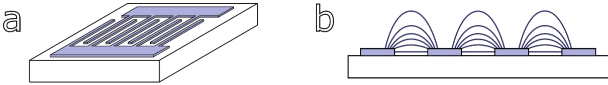
Figure 2.7. a) MSM interdigitated electrode geometry with b) electric field lines, device shown from the side.
