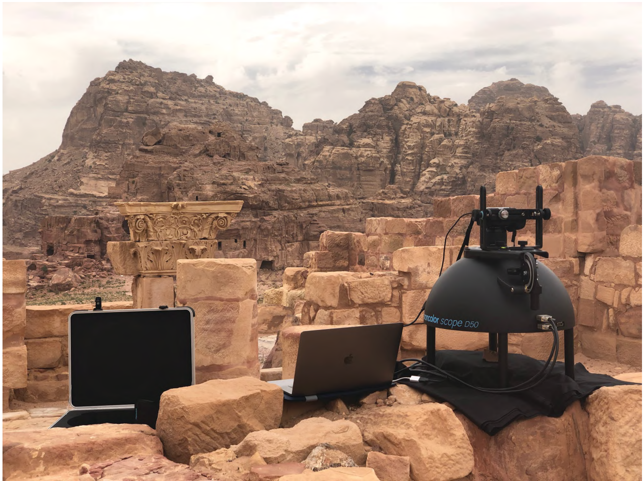
FIG. 3 Light dome with 48 white-light LEDs for capturing reproducible RTIs. Ez-Zantur (Petra, Jordan). (Photo by P. Fornaro.)
