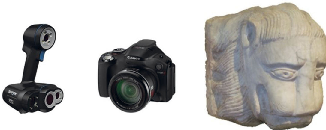
Figure 4. Structured light 3D scanner Creaform GO!Scan50 (left) and DSLR camera Canon PowerShot SX30 IS (centre). Test case: italic marble lion's head, "Doccione di fontana" (right), Galleria Nazionale dell'Umbria di Perugia, Italy.
